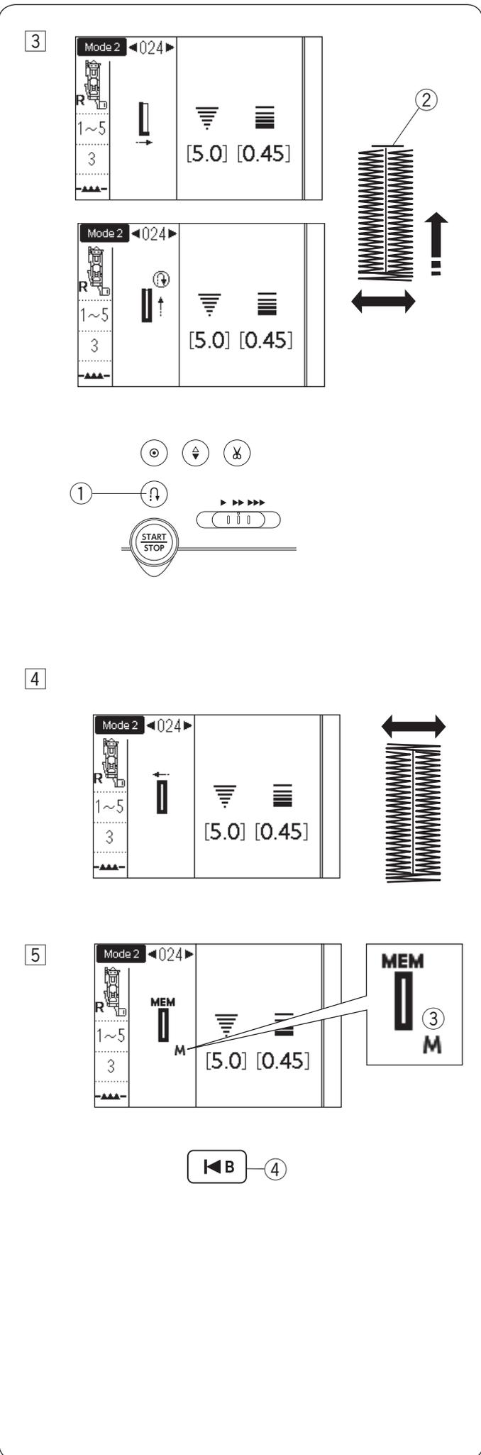
3 Start sewing again, and the machine sews the front bartack and right side of the buttonhole. Stop the machine when you reach the ending point (2). Then press the reverse key (1).
