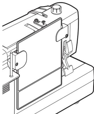
The back slots ① on the bracket are for store position. Slide stitch chart down between the back slots until the stitch chart stops.
