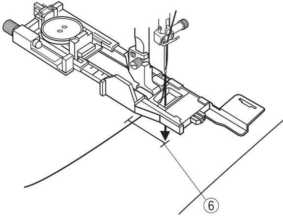
3 Draw the needle thread to the left through the hole of the foot.
