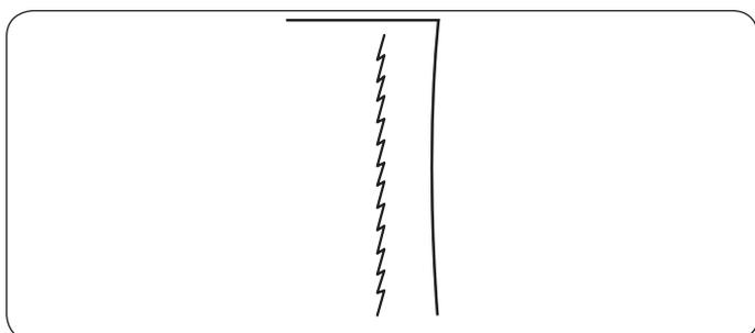
These are narrow stretch stitches designed to eliminate puckering on knit fabrics and bias seams, while permitting the seam to be pressed completely open flat.
