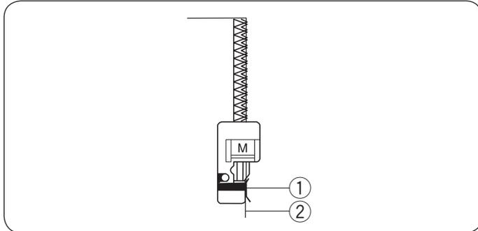
This is an excellent stitch for fabrics that tend to fray extensively such as linens and gabardines. Two rows of zigzag stitches are simultaneously sewn over the edge to insure that fabric will not ravel. Place the fabric edge next to the guide of the foot and then sew.
