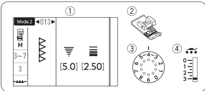
This stitch can be used to simultaneously seam and overcast edges of fabrics.
