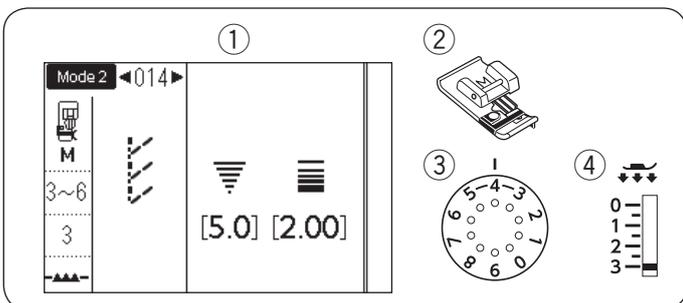
This stitch is recommended for sewing such fabrics as synthetic knits and stretch velour as it provides the greatest amount of elasticity and strength.
