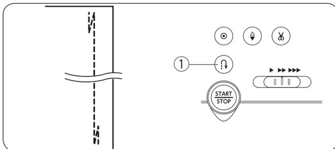
Use this stitch to secure the beginning and the end of a seam with backstitching.
