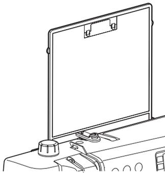
The front slots ② on the brackets are for view position. Pull up and out the stitch chart from back slots. Slide stitch chart down between the front slots.
