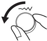
2 Turn the stitch width adjusting dial to adjust the width to "3.5".
