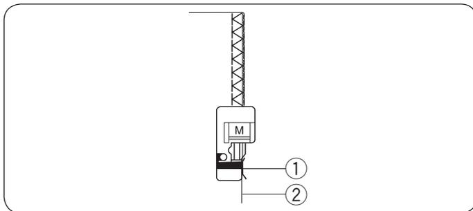
This stitch can be used to simultaneously seam and overcast edges of fabrics. Use this stitch when you do not need to open seams flat. Place the fabric edge next to the guide of the foot and sew.
