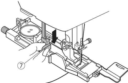
4 Lower the presser foot and pull the buttonhole lever down as far as it will go.
