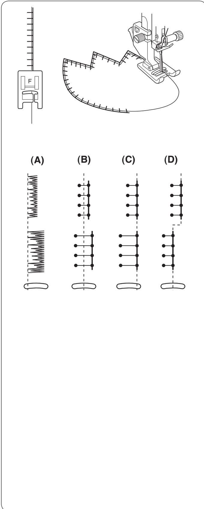
Place an applique on the fabric and baste it in place or use a fusible web to secure the applique in place. Guide the applique fabric, so that the needle falls off the edge of the applique when the needle swings to the right.
