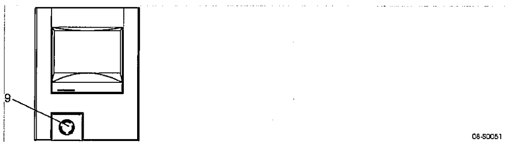
Fig. 17 Switching off in an emergency 9 EMERGENCY STOP pushbutton
