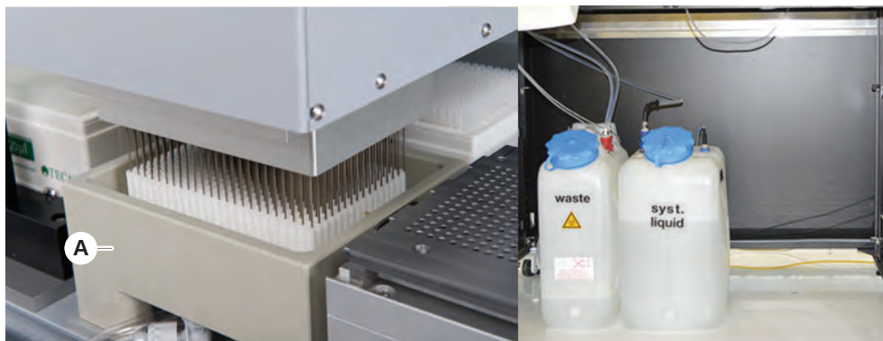
Fig. 28: Wash system (MCA)
