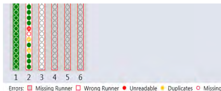
Fig. 40: Barcode reading confirmation displayed on the touchscreen
