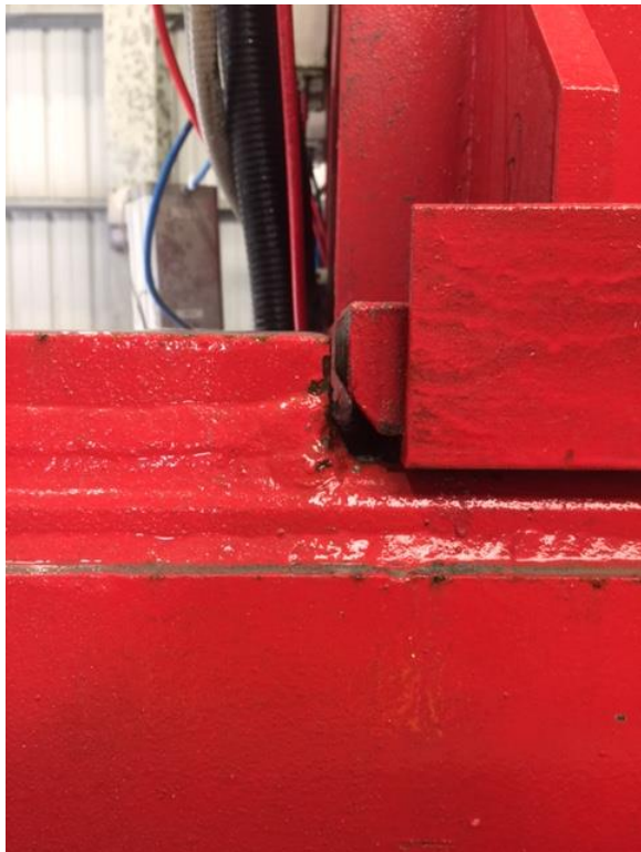
Plate out of alignment
