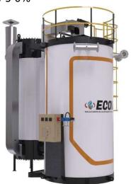
Vertical Type double concentric helical coil, three-steps, fully automatic type package with all accessories, complete and ready to work. Its exterior finish finished sheet of heat-resistant steel and is insulated with mineral wool and fire bricks.
