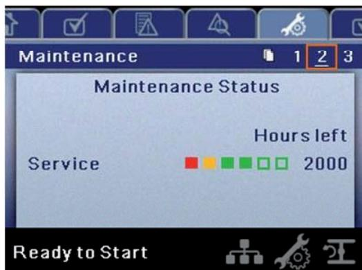
This page displays the time until the compressor should be serviced.
