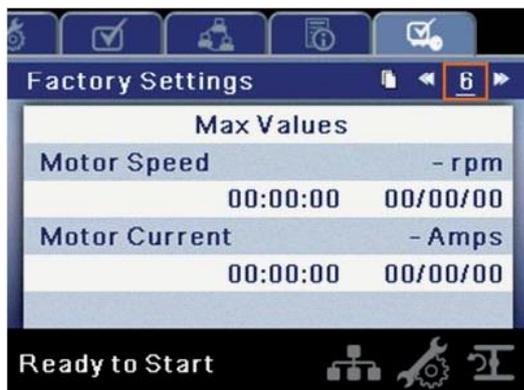
The maximum values pages are used to record the highest value the controller has seen since the last time the maximum values have been reset. Each maximum value entry displays the highest value recorded as well as the time and date stamp of when these maximum values have occurred.
