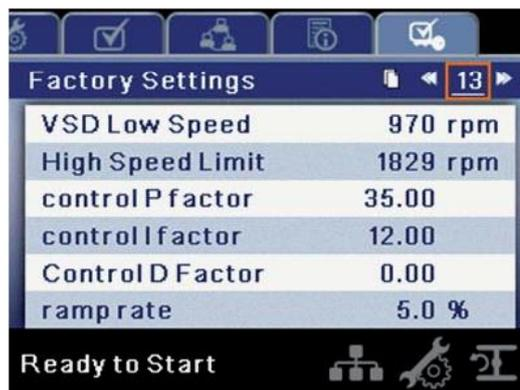
The VSD service menus contain parameters used to set up the compressor for optimal operation.
