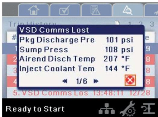
While the dialog box is active, press the left and right keys in order to scroll through the displayed data. The name of the trip will always be shown in the title bar of the dialog box. Press enter when finished viewing the data to return to the trip history screen.
