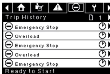
The pages in the Trips History folder document up to the last 15 trips that the controller has experienced, and time stamps each. The trips are recorded in sequence, with number one being the newest and 15 being the oldest. When a new trip occurs, it becomes number one and all others are shifted up in number.
