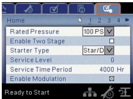
These pages are used for setting parameters that are specific to the compressor. All of the factory settings that are adjustable are listed below. All settings on these pages are password protected.
