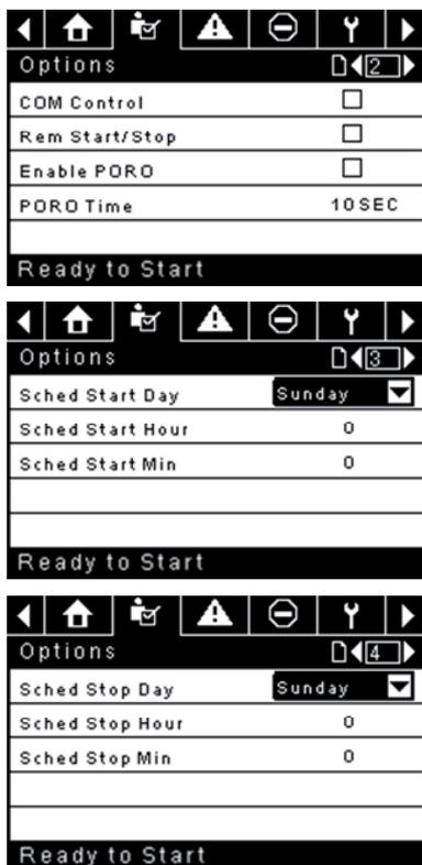
The options set points are similar to the operator set points except these set points cannot be changed while the unit is running.
