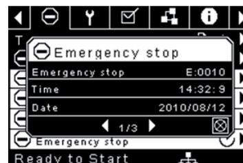
While the dialog box is active, press the left and right keys in order to scroll through the displayed data. The name of the trip will always be shown in the title bar of the dialog box. Press enter when finished viewing the data to return to the trip history screen.
