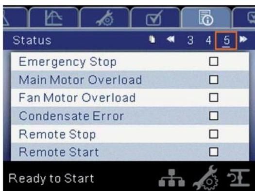
A marked checkbox beside a digital input indicates that the input is in its TRUE state. For example, Starter Feedback is TRUE when its input is in the high state, whereas, E-Stop is TRUE when its input is at 0Vdc.
