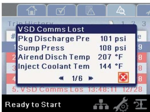
While the dialog box is active, press the left and right keys to scroll through the displayed data. The name of the trip will always be shown in the title bar of the dialog box. Press enter when finished viewing the data to return to the trip history screen.
