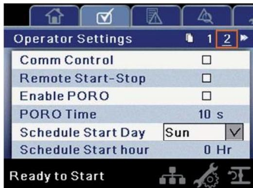
The parameters immediately below are only adjustable when the compressor is stopped.
