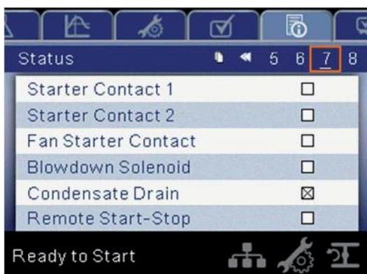
A marked checkbox beside a digital output indicates that it is energized.
