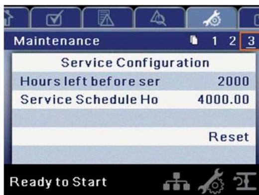
This page allows the user to set the service interval and to reset the counter after the service has been performed.
