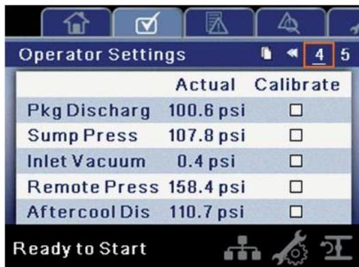
Sensor calibration can only take place when the compressor is stopped. There should be no pressure on a sensor when it is calibrated. Calibration only needs to take place after a sensor is replaced, the controller is replaced, or the operator suspects the sensor reading is in error. Calibrate a sensor by selecting the checkbox beside the sensor name.
