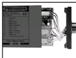
Picture 2. After this, the back panel can be pulled out together with the PCB, but please notice the position of the PCB as there is a number of different positions in the house. Do not pull the wires unnecessarily, instead pull the PCB. Switches and jumpers can now be moved. When assembling the back plate and housing, please make sure no wires are stuck.
