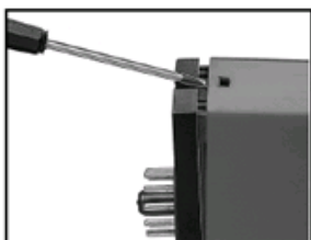
Picture 1. The back panel of the module is detached from the housing by way of a screwdriver.
