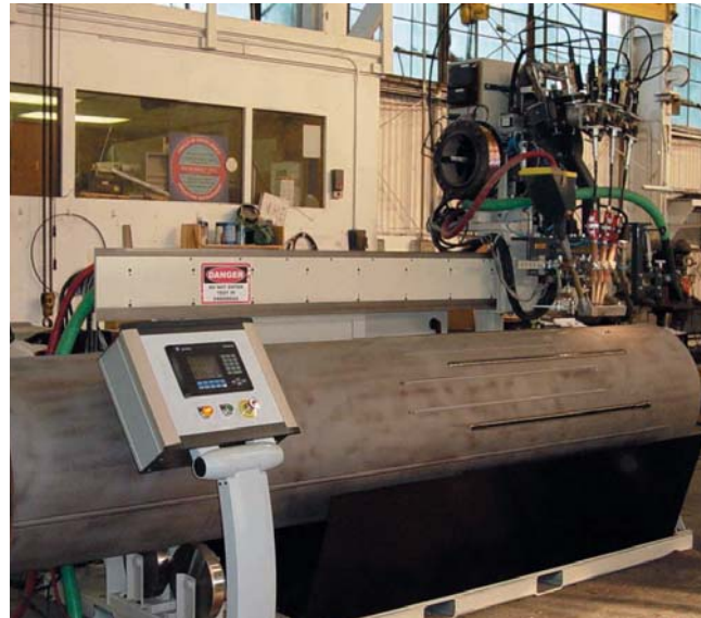
Three-Arc AC/DC Submerged Arc welding system controlled by a PLC
