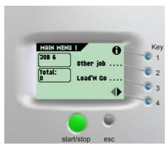
Press the start/stop key to start the machine. When the start/stop key is pressed again the machine stops feeding after completing the set. It is possible that there are still documents left in the document feeder (for example a small card). Remove all these documents from the feeder before restarting another job. There can also be envelopes left in the envelope track. These envelopes must be removed when another type of envelopes is required.
