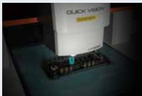
Example of measuring an engine control unit
