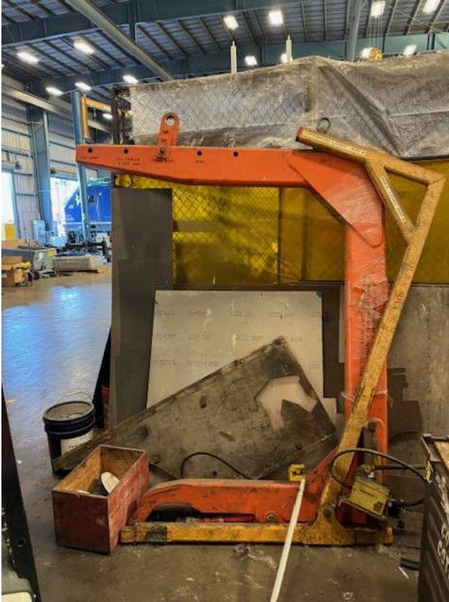
C-Clamp Lifting Device (7'6" x 3.5" x 6')
