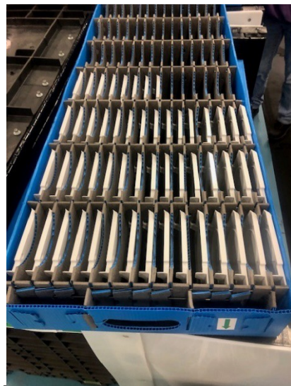
Tray C Dimensions (Blue): 7" tall, 16" Wide, 42" Long (inner compartments 7.5" x 4")
