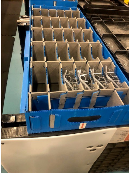
Tray E Dimensions (Green): 7.5" Tall, 16" wide, 42" long (inner compartments 2" x 3")
