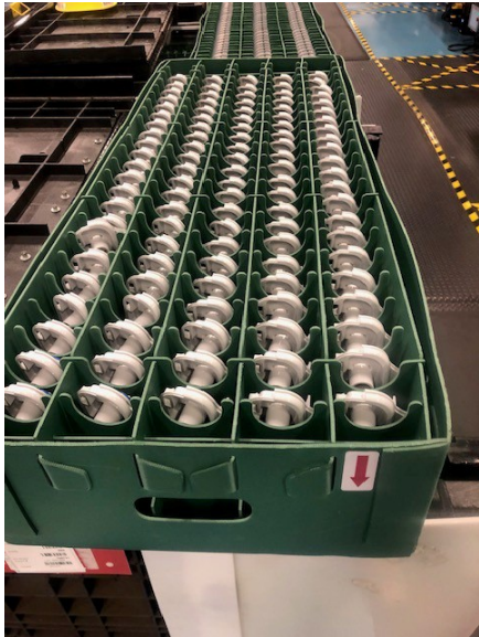
Tray F Dimensions (Green): 4.5" Tall, 16" Wide, 42" long (inner compartments 2" x 5")
