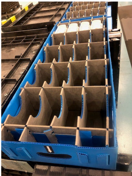
Tray C Dimensions (Blue): 7" tall, 16" Wide, 42" Long (inner compartments 7.5" x 4")
