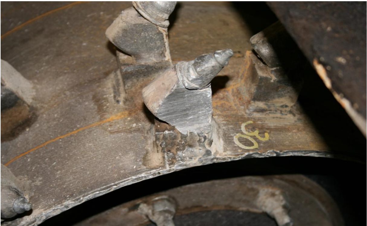
Tooth is no longer rotating in the holder, causing premature tooth and holder wear.
