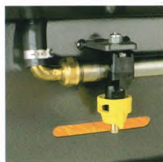
Sprinkler system - the water is injected into the brush roller from behind to minimize dust and save water.
