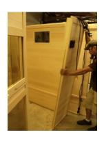
The Front is separated into Two pieces. One has the door, the other has the timer/control.
