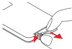
2. Install new battery into the compartment. Remove the old battery and install new one (CR2025). Ensure that the side with a "+" is facing up.
