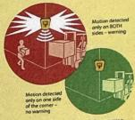
The Collision Sentry Corner Pro sends a warning ONLY when it senses movement in both detection zones; motion on both sides of the blind corner.
